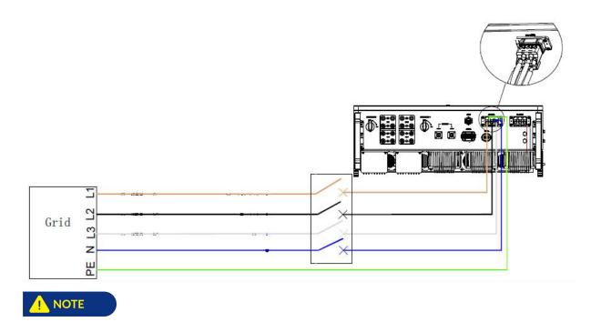
Install a circuit breaker between the power grid and the PCS. Please note that AlphaESS does not provide this circuit breaker. If a circuit breaker is installed, there is no need for a leakage protector between the power grid and the PCS.
