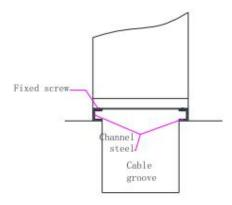
When the STORION-G2-H30/H50-O outdoor cabinet needs to be fixed to the concrete floor, holes need to be drilled into the floor and screws should be used to secure the cabinet. Connect the grounding point at the bottom of the rear door of the STORION-G2-H30/H50-O outdoor cabinet to the on-site grounding point using a grounding wire, and tighten it with bolts after connection. The schematic diagram for fixing the cabinet to the concrete floor is shown below:
