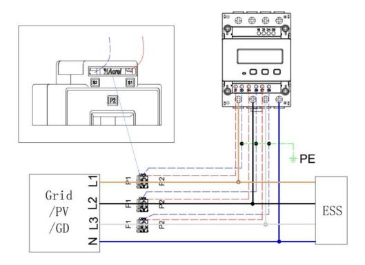
The positive direction corresponding to the positive value of the energy storage meter data is defaulted as shown in the preceding figure. The meters installed by STORION-G2-H30/H50-O include grid gateway meters, PV grid connection point meters, and diesel electromechanical meters.
