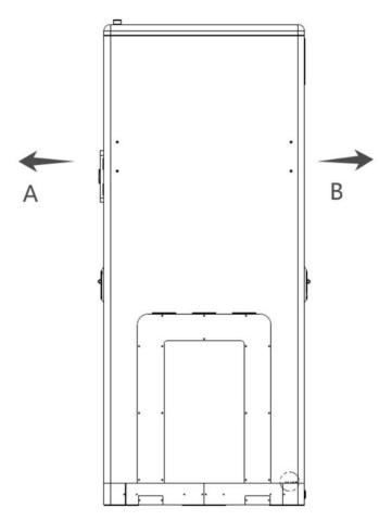
A  $\geq$  1300 mm: Ensure that the front door of the cabinet can be fully opened, allowing for proper ventilation and heat dissipation, as well as sufficient space for operation and maintenance.
