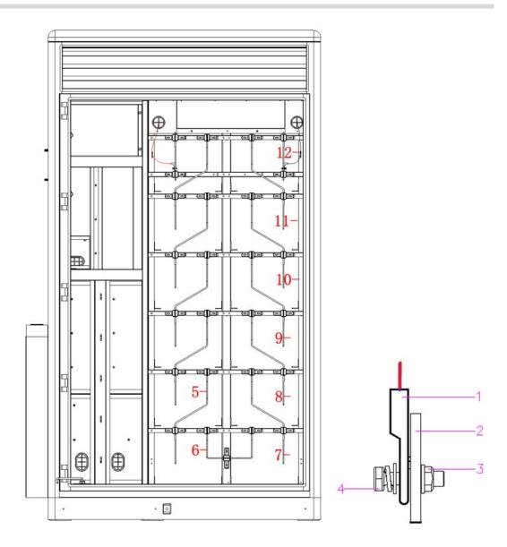
The wiring harness and copper bar connection configuration are described in the following table:
