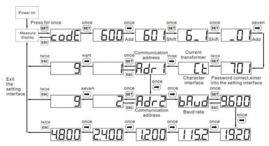
According to this step, the baud rate can be checked and the communication address can be set. The corresponding communication addresses and baud rates for each meter are as follows:
