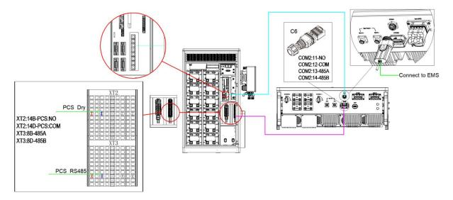
1. Connect the PCS to the outdoor cabinet debugging communication harness, and use the reserved harness to connect the PCS COM2 (COM2:13/COM2:14) to the outdoor cabinet terminal block (XT3:8B/XT3:8D) (already wired).
