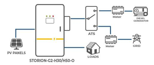
The schematic diagram of parallel operation is as follows:
