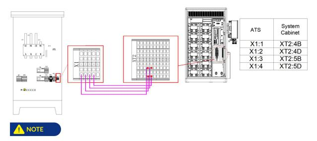
The dry contact voltage is 24V. It is recommended to use a 2-core shielded twisted pair cable with a cross-sectional area of 0.75m<sup>2</sup> or more.
