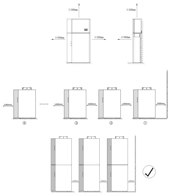
Recommended clearances for series batteries SMILE-G3-BAT-3.6S/3.8S/4.0S. It's advisable to keep the series batteries at least 150mm off the ground to protect them from submergence. They should be mounted on a battery base or using a wall bracket.
