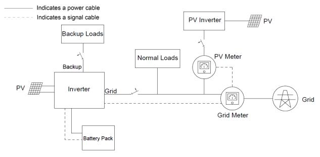
Brief wiring diagram of the hybrid-coupled system
