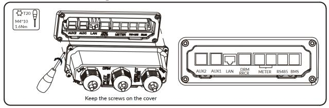
2. Pass the communication cables through the cable glands of the COM connection cover. Do not tighten the strain relief nuts of the cable glands yet.
