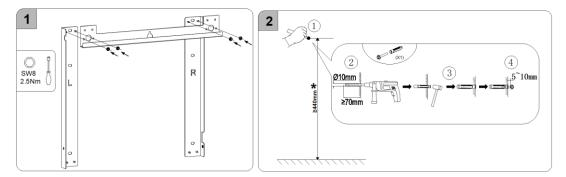
\* This recommended value "440mm" is for wall bracket location of the bottom battery. Depending on the number of expansion batteries mounted later, meanwhile it is advisable to have a minimum of 150~200mm off the ground to protect the system from submergence.
