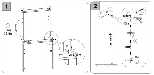
\* This recommended value "870mm" is for wall bracket location of the second battery seeing from the bottom up. This value may adjust depending on the number of expansion series batteries mounted later.
