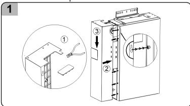
Disassemble the cable cover of the battery SMILE-G3-BAT-8.2P
