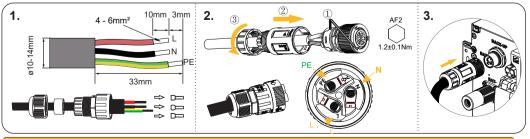
The wiring steps are only suitable for backup connection of SMILE-G3-S5/S3.6/B5-INV.
