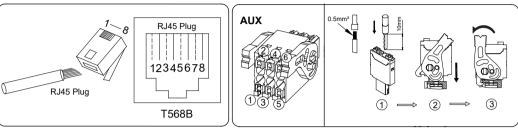
5.3 Wiring the Communication Cables between the Inverter and Battery
